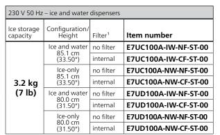
Internal filter is a 5 micron particle and carbon filter
