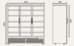
Gross volume: 1260 L Exterior dimensions in mm: 1875w x 730d x 2000h Number of adjustable shelves: 15 Temperature set range:  $0^{\circ}$ C to  $+6^{\circ}$ C Gross/net weight: 225/210 kg Energy consumption in 24h: 11.5 kWh
