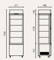
Temperature set range:  $+2^{\circ}$ C to  $+12^{\circ}$ C Gross/net weight: 80.5/76.4 kg Energy consumption in **24h**: 5.46 kWh
