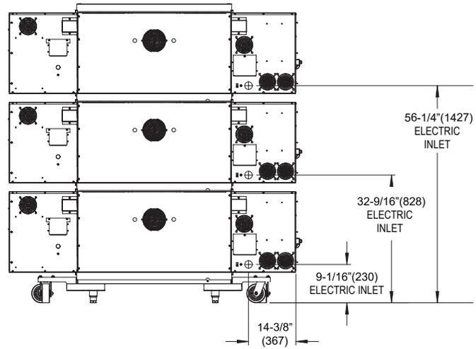
PS640 Back View – Electric Triple Stacked w/Outriggers
