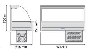
Note: For CRX model range overall height dimensions, add height of motor cage (450 mm).
