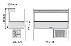
Note: For SRX model range overall height dimensions, add height of motor cage (450 mm).
