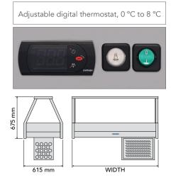
Note: For ERX model range overall height dimensions, add height of motor cage (450 mm).
