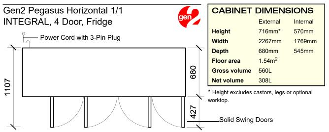
Side Mounted Integral Refrigeration Unit Electronic
