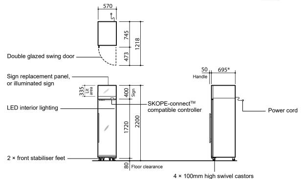
CABINET Model ID SKT500XW SKT500XW-CX SKT500XW-C 1 × self-closing, reversible, double glazed, single Low-E, lockable, argon Doors filled, toughened safety glass swing door (hinged RH) 1 × door openings: 1570mm high × 450mm wide Internal door opening Shelves 5 × adjustable height wire shelves: 445mm wide × 470mm deep Sign Sign replacement panel Illuminated sign Material Powdercoat galvanized steel or stainless steel interior & exterior
