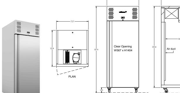
**SPECFICATIONS CAPACITY LITRES** 610 TEMPERATURE -18°C / -22°C DIMENSIONS - W X D X H (ON 120 727 W x 824 D x 1974 H MM H CASTORS) MM WEIGHT UNPACKED (KG) 170 STANDARD INCLUSIONS \*\*\* Standard: S (Solid Door) DOOR TYPE FINISH (INTERIOR AND EXTERIOR S (Stainless Steel) **EXCLUDING REAR AND UNDER)** SHELVES/DOOR (ADJUSTABLE 4 **STRIPS AND CLIPS)** GAS TYPE R290 REFRIGERANT
